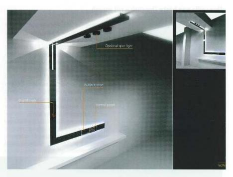
for interiors which adapts to walls, corners, ceilings and pendants. The modules fit together like segments and permit one single design for lighting, sound, time and weather. The light fittings, made in varnished or anodized aluminium extrusion, adopt fluorescent sources, with one-colour or RGB LED strips; LED, halogen or HQI projectors can also be fitted and hung in any position right along the system. An
